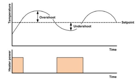
Figure 7 Response of an on-off control system
