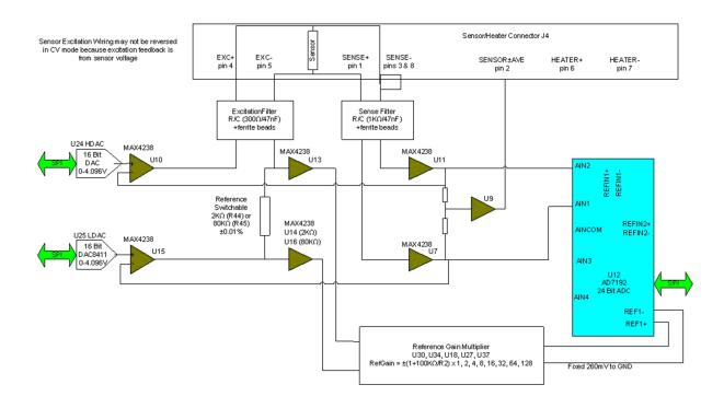
The sensor and a reference resistor (either R44 or R45) are connected in series. Digital to analogue converters U24 and U25 generate an upper and lower demand voltage. The upper voltage is buffered by U10 and applied to the upper end of the sensor resistor. The lower
