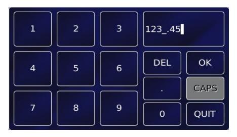
The keypad has a parameter box in the top-right corner that displays the number that been entered so far.
