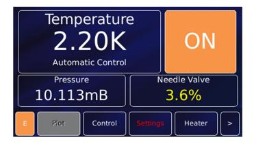
In automatic control the user cannot set the needle valve opening. Now control is determined by the internal algorithm forming the key part of the LPF control. In this mode the LPF will attempt to cool the LPF to a temperature as close as possible to 2.20K by adjusting the flow through the LPF based on the LPF pressure signal for control feedback. There is a defined sequence of steps, which are indicated by the status message, and there are 3 "zones" of operation.
