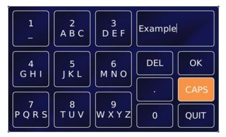
The keypad has a parameter box in the top-right corner that displays the text that has been entered so far.
