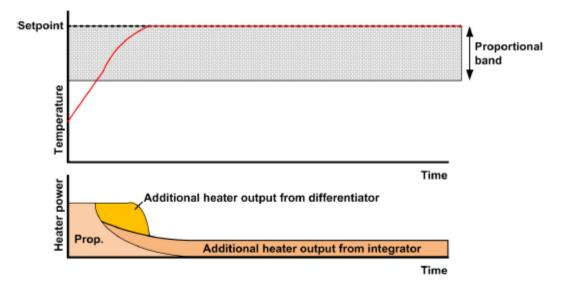
Figure 10 Proportional control with integral and differential action
