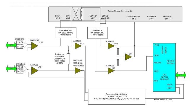
The sensor and a reference resistor (either R44 or R45) are connected in series. Digital to analogue converters U24 and U25 generate an upper and lower demand voltage. This voltage is equal to the required current multiplied by the value of the selected reference resistor.
