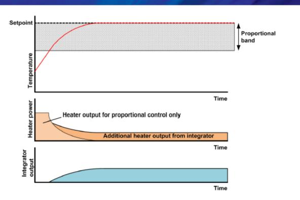
Figure 9 Proportional control with integrator action
