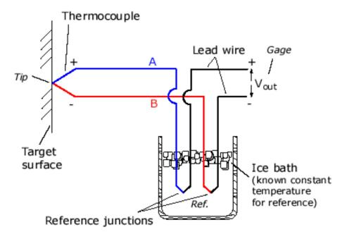
The simple diagram above shows the use of an ice bath to maintain the temperature of the reference junctions. A calibration file with a zero voltage at the ice point must be used.
