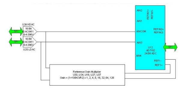
The calibration is performed using a ratiometric circuit configuration. In calibration mode, DACs U24 and U25 supply a differential calibration voltage to the input of ADC U12. This same differential voltage is scaled by a reference gain multiplier circuit and supplied to the reference voltage inputs of U12.
