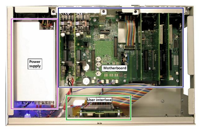
Figure 3 View of internal layout of MercuryiTC
